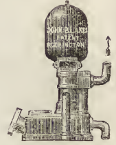
This Ram will force up spring water whilst worked by impure water.
